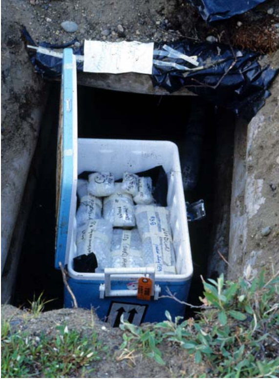
Cooler in cold storage pit dug into permafrost .
