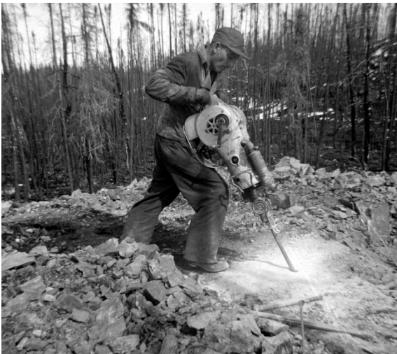
Diamond driller surface drilling at Hottah Lake with hand-held drilling machine.
